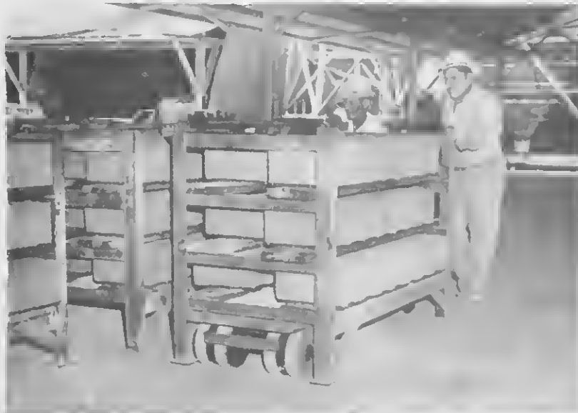
NEW BLOCKS must be kept under cover for several hours to allow them to set up. As soon as a pallet has been filled it is moved from the press to storage (above).
